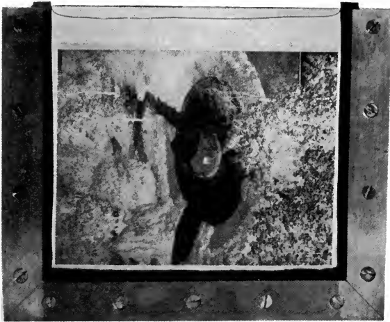
FIG. 4. Thin water cell for holding wet cut films in the enlarger.
